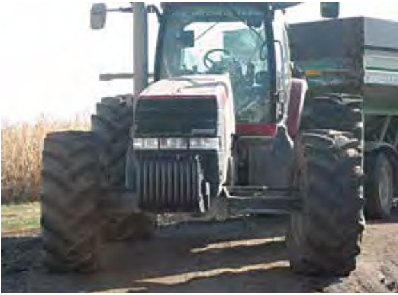
Figure 15.10. A tractor with wide wheel spacing to fit a controlled traffic system.
