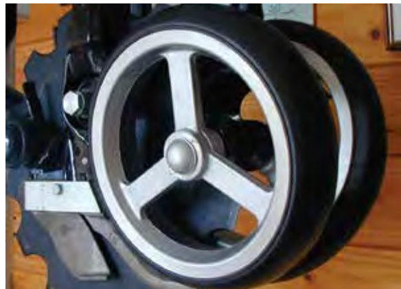
Figure 16.8. Left: A no-till seed drill requires no-till or seedbed preparation for narrow-seeded crops or cover crops. Right: The cross-slot opener used in no-till planters. The disk slices soil, the inverted T blade allows seed and fertilizer placement on opposite ends of the disk, and the packer wheels (right side) close and firm the seedbed.
