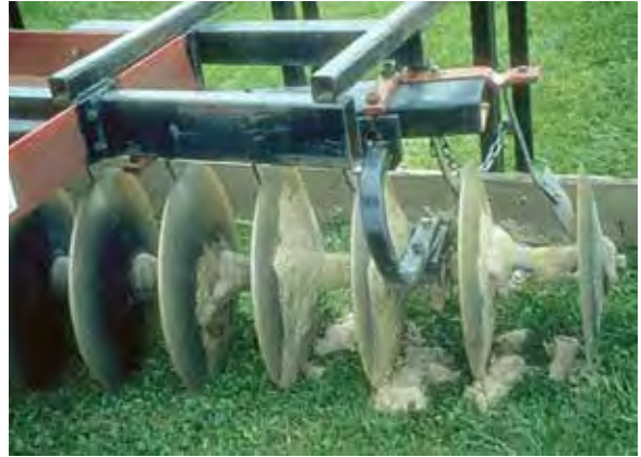
Figure 16.5. Left: A heavy disk (disk plow) can be used for primary and secondary tillage. Photo by Mark Brooks. Right: A finishing disk.
