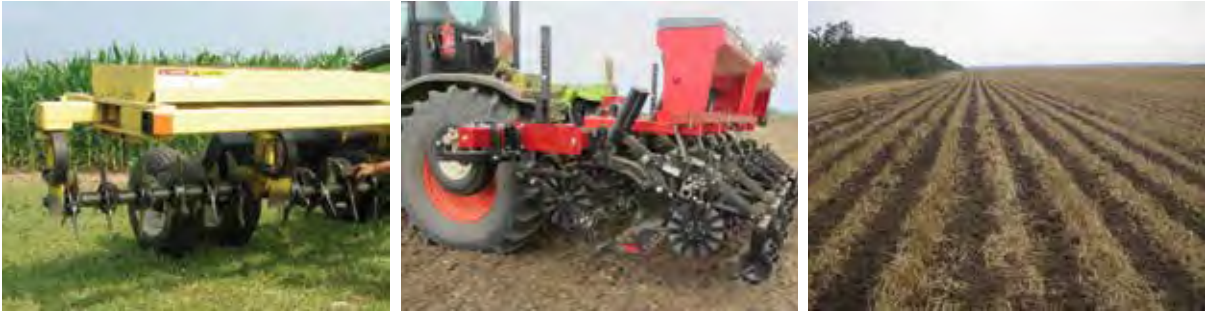
Figure 15.4. Tools that provide compaction relief with minimal soil disturbance: aerator (left) and strip tiller (middle and right). Right photo by Georgi Mitev.
